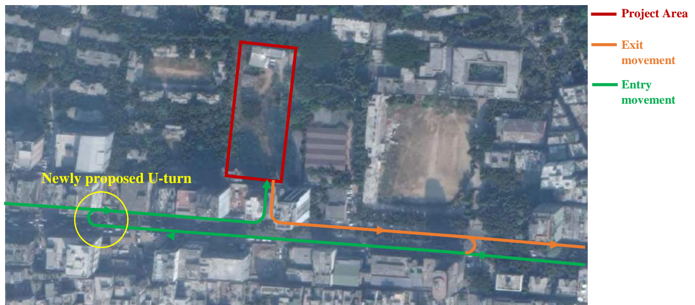
Figure 6.10: Traffic circulation on the link and access roads of the project site as proposed in the present study (considering phase-1 only)
